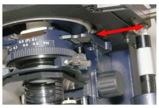
Figure 13. Insertion of the dark-field ring
