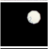
3. Move the condenser up or down so that the diaphragm edges are in focus. The microscope is designed so that in the imaging path, field diaphragm should be in conjugate plane with the specimen plane (in focus at the same time). You adjust this by adjusting the height of the condenser.
