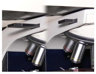
Figure 10. Analyzer for polarization contrast imaging
