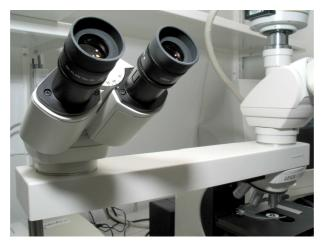
Figure 7. Dual viewing attachment
