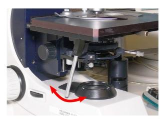
Figure 4. Auxiliary condenser lens switch
