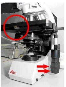
Figure 2. Adjustment wheels for stage control (arrows) and rotation lock (circle)
