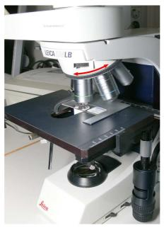
Figure 3. Objective revolver (red arrow) and sample holder
