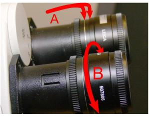
Figure 6. Diopter adjustment. A, setting for 0 diopter; B, diopter adjustment
